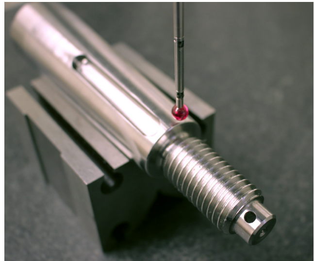
CMM inspection on shaft tapers to verify precision accuracy.
